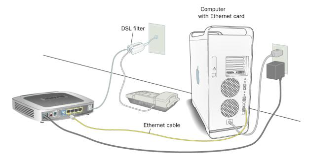
Figure 7. Gateway Connected Via Ethernet (Macintosh)
